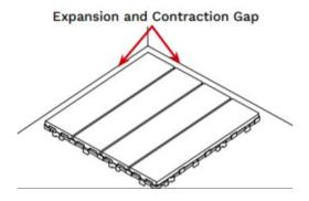
Areas above 9m in length must also have a break in the layout of 5mm to allow for expansion and contraction and avoid warping. The tiles simply connect together with the fittings provided as part of the tile as shown below.
